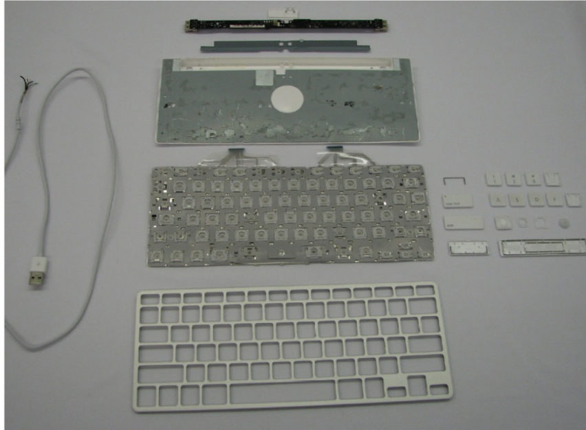
Figure 5.2: Keyboard After Disassembly
